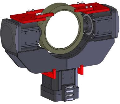
Figure 1-2: Lifting Features
