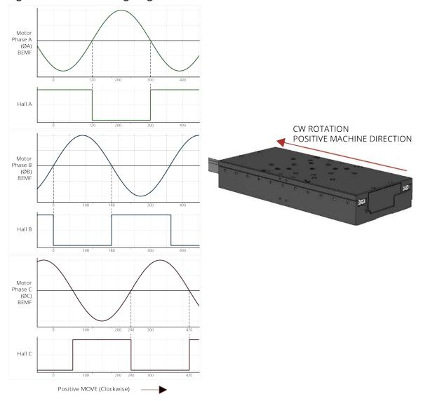
Figure 3-5: Encoder Phasing Reference Diagram (Standard/Square Wave)
