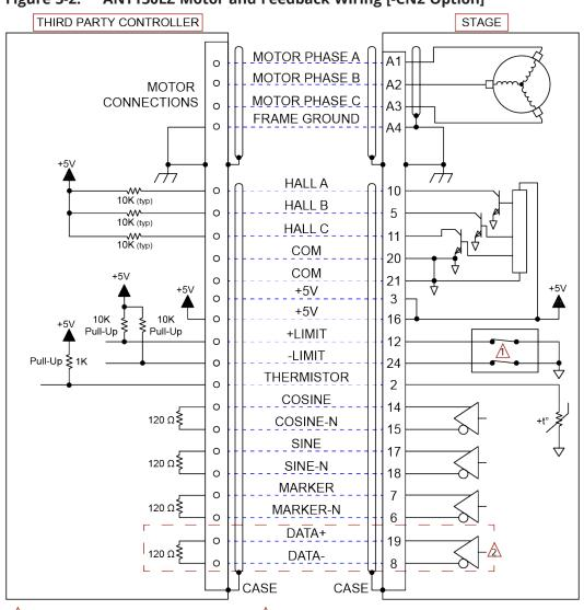
Figure 3-2: ANT130LZ Motor and Feedback Wiring [-CN2 Option]
