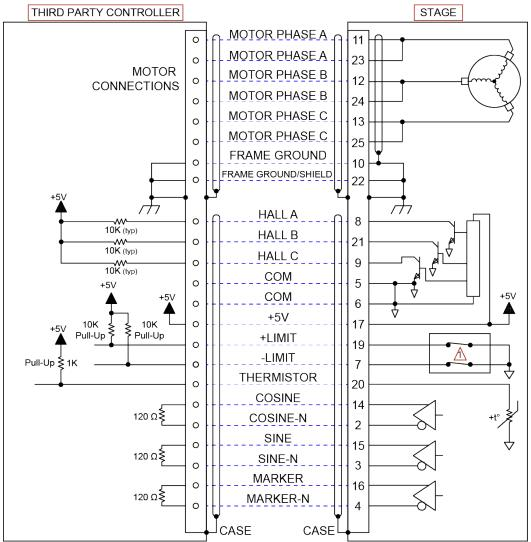
$\bigwedge$  Over-travel limit switches are normally-closed.
