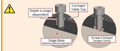
Applied loads should be symmetrically distributed whenever possible. The payload should be centered on the stage mounting surface and the entire stage should be centered on the support structure.
