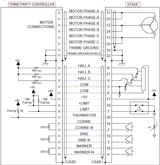
$\bigwedge$  Over-travel limit switches are normally-closed.
