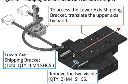
Figure 5: Shipping Bracket Removal Procedure (Step 2)
