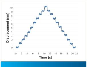
ANT95LZS-025-PL2 1 nm step plot. Best-in-class resolution and exceptional in-position stability for large-travel stages.
