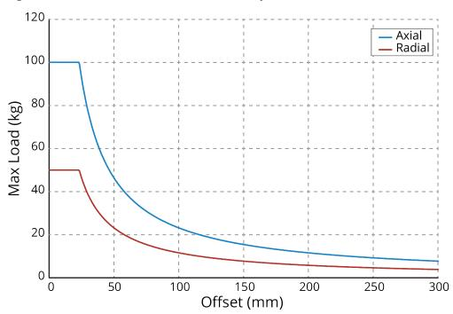
Figure 2-14: AGR100 Cantilevered Load Capabilities
