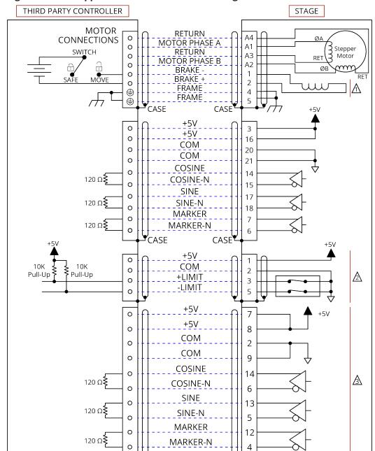
Figure 3-3: Stepper Motor and Feedback Wiring
