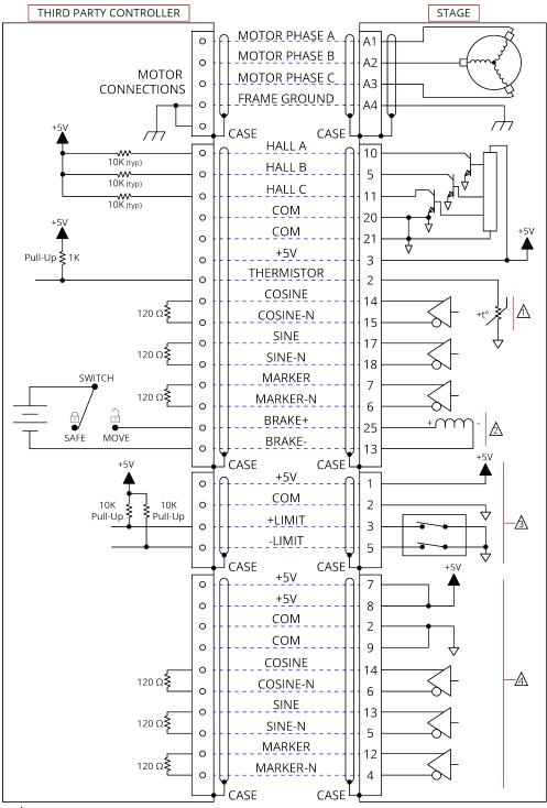
Thermistor is only available on BMS motors (options -M1, -M2, -M3, and -M4).
