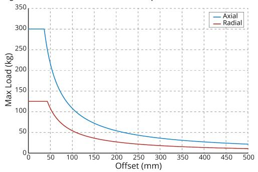
Figure 2-16: AGR200 Cantilevered Load Capabilities
