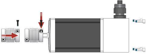
6. Attach the Motor to the Stage in the correct orientation (Figure 4-4). Use a hex wrench to ensure that the motor flange is fully seated and the hardware is tight. The motor housing prevents the use of a torque wrench.
