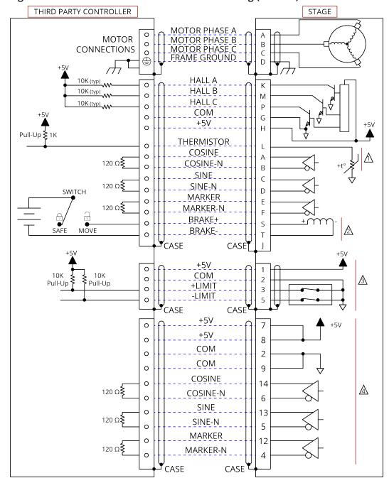
Figure 3-2: Brushless Motor and Feedback Wiring (AGR200)
