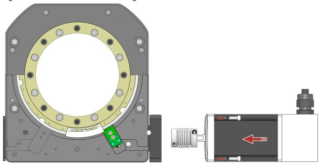
7. Tighten the Shaft Coupling to the drive screw (Figure 4-5). Refer to Table 4-1 for the correct hardware and torque requirements.
