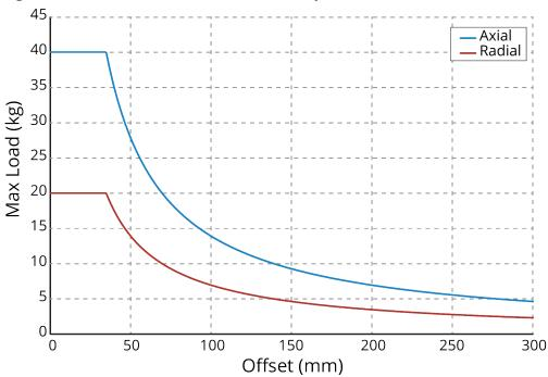
Figure 2-13: AGR75 Cantilevered Load Capabilities
