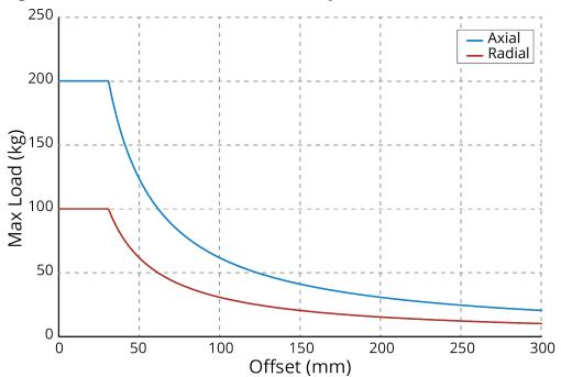
Figure 2-15: AGR150 Cantilevered Load Capabilities
