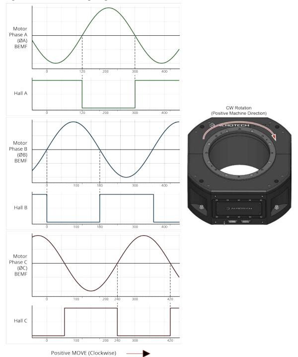
Figure 3-6: Encoder Phasing Reference Diagram (Standard/Square Wave)
