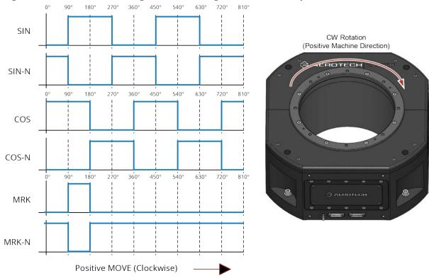
Figure 3-7: Encoder Phasing Reference Diagram (Analog/Sine Wave)
