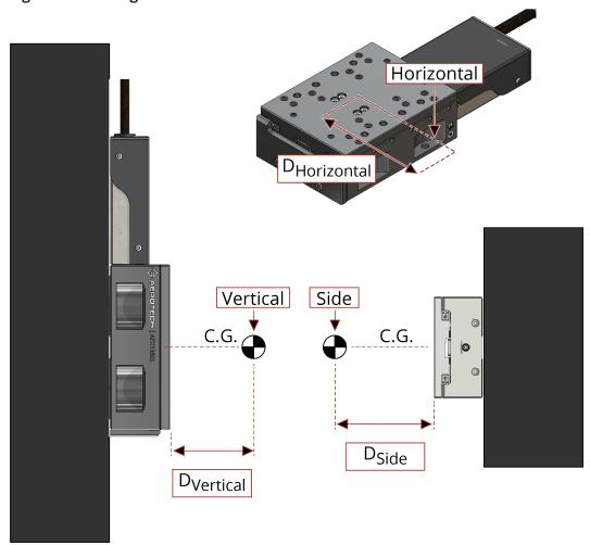
Figure 2-6: Cantilevered Load Capability
