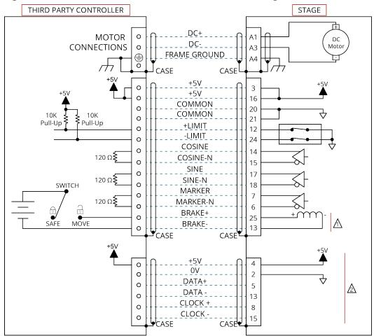
Figure 3-3: ATX115SLE-E3 DC Motor and Feedback Wiring
