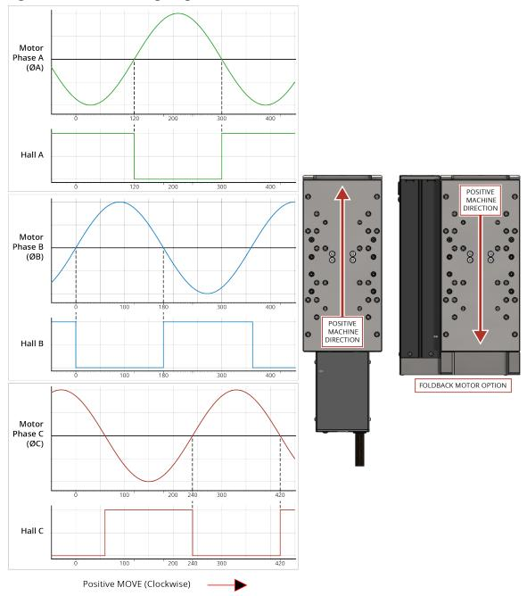
Figure 3-9: Encoder Phasing Reference Diagram (Standard/Square Wave)
