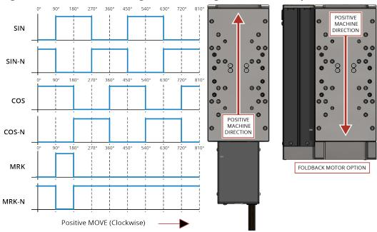
Figure 3-10: Digital Encoder Phasing Reference Diagram (Sine Wave)
