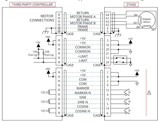
Figure 3-5: ATX115SLE-E1 and -E2 Stepper Motor and Feedback Wiring
