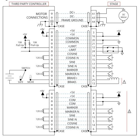
Figure 3-2: ATX115SLE-E1 and -E2 DC Motor and Feedback Wiring
