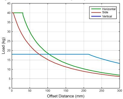
Figure 2-7: Cantilevered Load Capability
