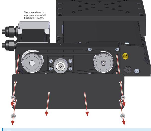
**IMPORTANT**: If the stage has been calibrated (-PL2 option), note the orientation of the two pulleys with regard to each other or recalibration might be required.
