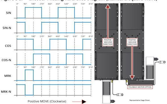
Figure 3-5: Encoder Phasing Reference Diagram (Standard/Square Wave)
