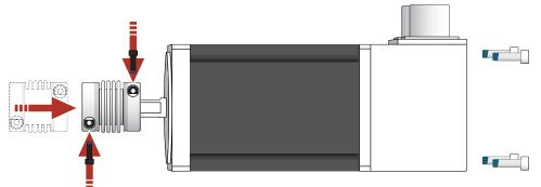
6. Attach the Motor to the Stage in the correct orientation (Figure 4-6). Use a hex wrench to ensure that the motor flange is fully seated and the hardware is tight. The motor housing prevents the use of a torque wrench.
