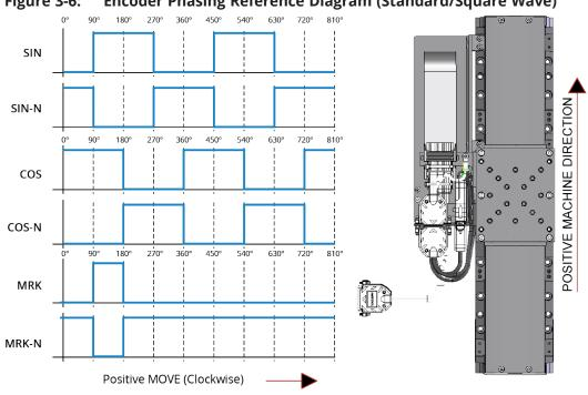
Figure 3-6: Encoder Phasing Reference Diagram (Standard/Square Wave)
