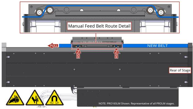
Figure 4-8: Manual Feed Method
