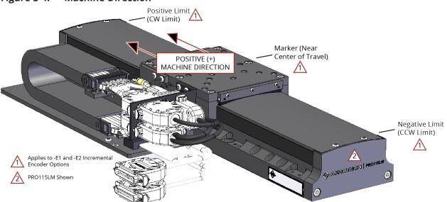
Figure 3-4: Machine Direction
