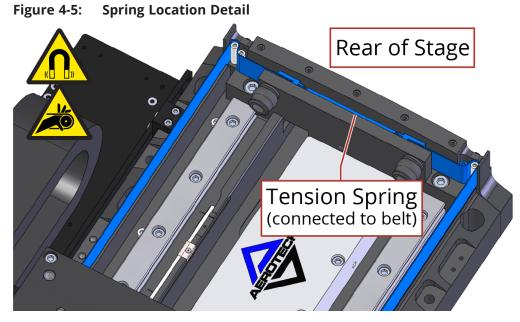
There are two methods that you can use to install the new belt through the stage table: **Pull Through Method**: Use this method if the old belt is intact and fed through the stage table. **Manual Feed Method**: Use this method if the old belt is not fed through the stage table.
