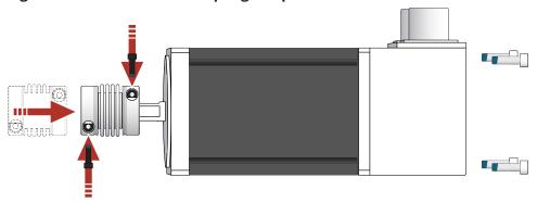
6. Attach the Motor to the Stage in the correct orientation (Figure 4-6). Use a hex wrench to ensure that the motor flange is fully seated and the hardware is tight. The motor housing prevents the use of a torque wrench.
