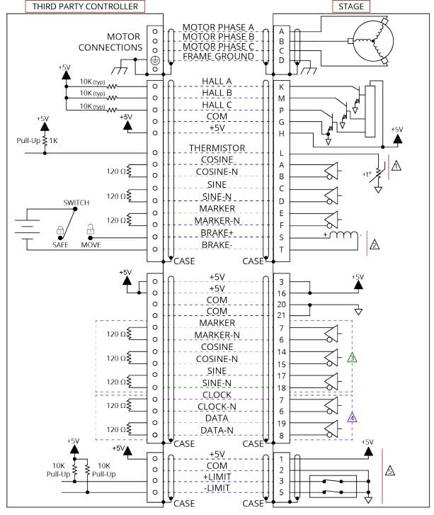
Figure 3-2: Brushless Motor and Feedback Wiring [-SLE Option]
