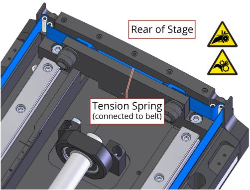
There are two methods that you can use to install the new belt through the stage table: **Pull Through Method**: Use this method if the old belt is intact and fed through the stage table. **Manual Feed Method**: Use this method if the old belt is not fed through the stage table.
