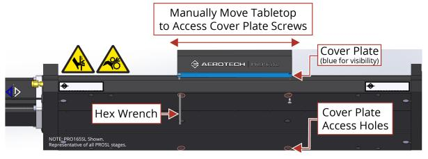
Figure 4-12: Manual Feed Method
