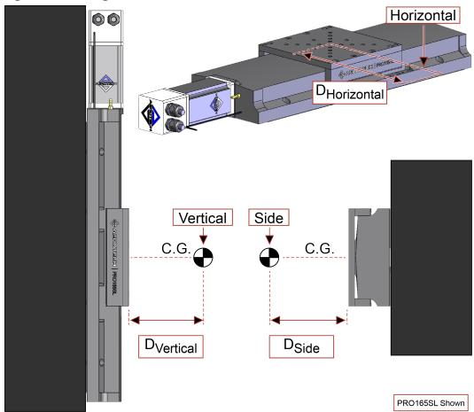
160 Horizontal Side 140 Vertical 120 100 Load (kg) 80 60 40 20 0 50 100 150 200 250 300 Offset Distance (mm)
