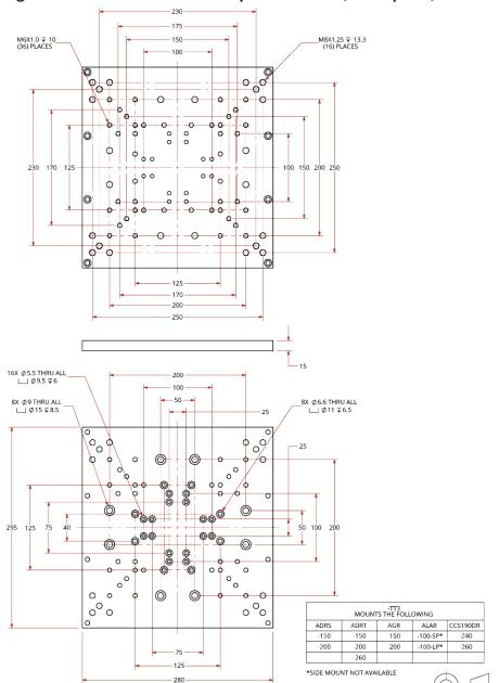
Figure 2-4: PRO280SLE Tabletop Dimensions (-TT3 Option)
