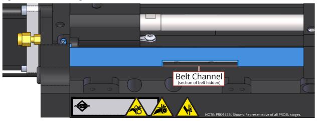
12. Once the belt is fully adjusted, trim the ends of the belt as shown in Figure 4-15.
