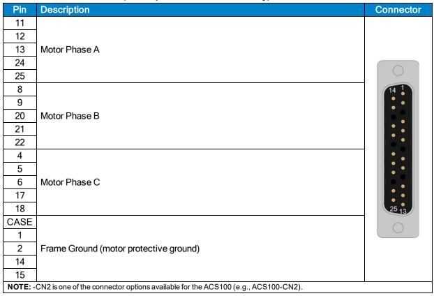
Table 3-4: Mating Connector Part Numbers for the -CN2 Motor Option Connector
