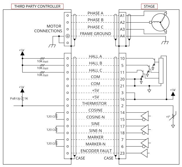
Figure 3-3: Motor and Feedback Wiring (ACS150 and ACS200)
