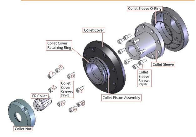
Figure 2-9: Collet Assembly Exploded View
