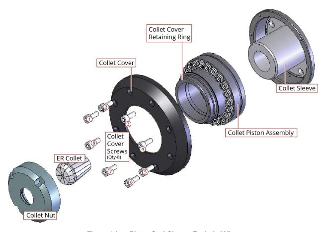
Figure 4-1: Piston Seal Change Exploded View
