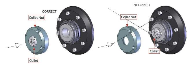
Figure 2-8: Installation Procedure for Collet
