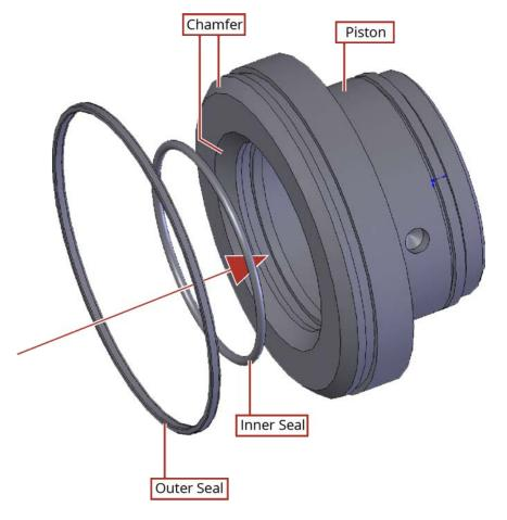
Figure 4-2: Piston Seal Installation Procedure
