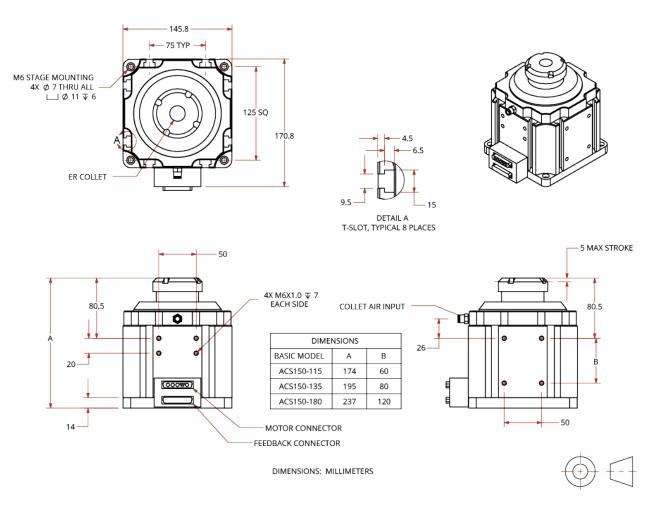
Figure 2-2: ACS150 (-ER Chuck Style) Dimensions
