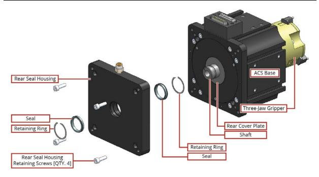
Figure 4-4: Exploded Drawing of Rear Seal Components
