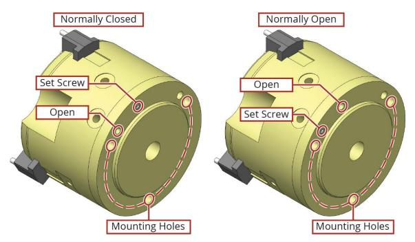
Figure 2-12: Air Inlets in Three-Jaw Grippers
