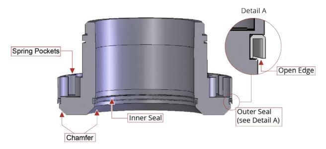
Figure 4-3: Cross-Section View of Piston Showing Seal Orientation
