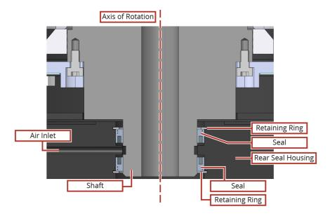
Figure 4-5: Cross-section View of Rear Seal Showing Seal Orientations
