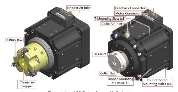
Figure 1-1: ACS Rotary Stage with Callouts
