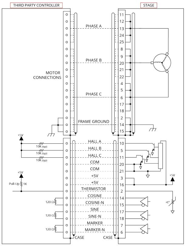
Figure 3-2: Motor and Feedback Wiring (ACS100 -CN2)
