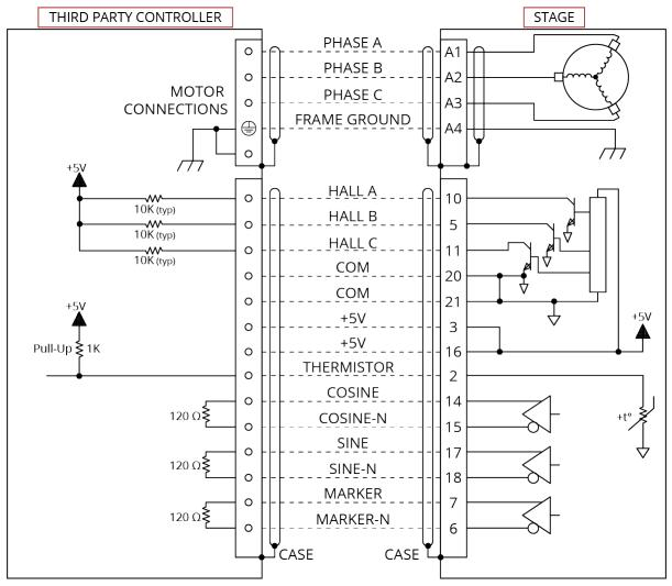
Figure 3-1: Motor and Feedback Wiring (ACS100 -CN1)
