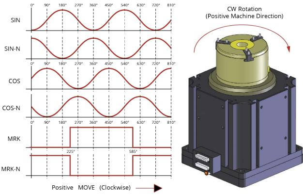
Figure 3-6: Analog Encoder Phasing Reference Diagram
