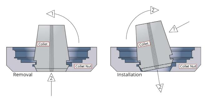
Figure 2-7: Schematic of Collet Insertion Into and Removal From Collet Nut
