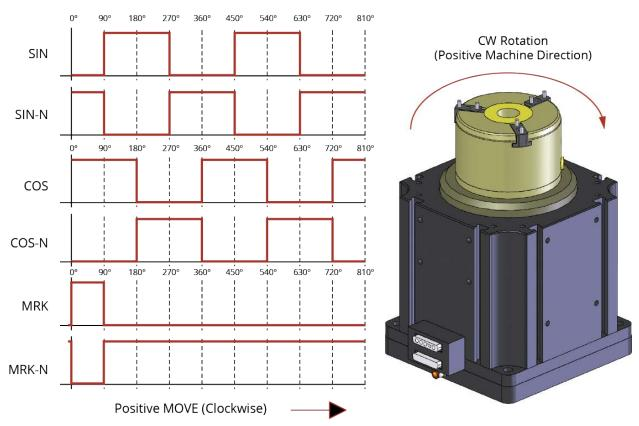
Figure 3-7: Encoder Phasing Reference Diagram (Standard)
