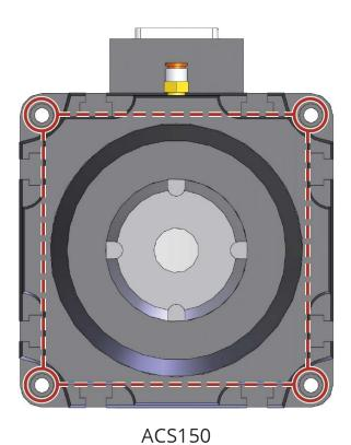
Figure 2-5: ACS Stage Mounting Holes
