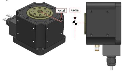
Figure 2-4: Cantilevered Load Capabilities
