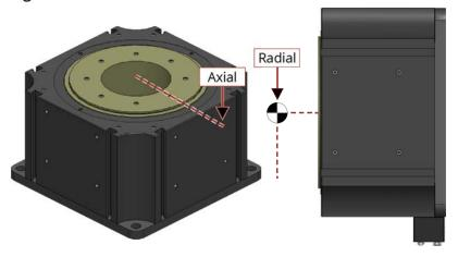
Figure 2-5: Cantilevered Load Capabilities
