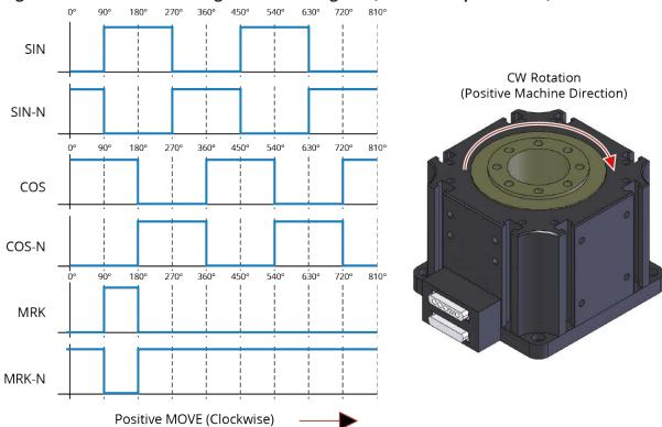
Figure 3-4: Encoder Phasing Reference Diagram (Standard/Square Wave)
