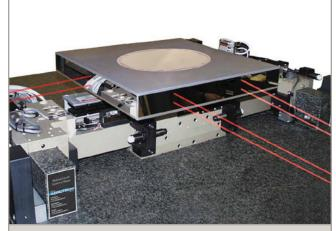
Multi-axis interferometer feedback is available to control X and Y position, as well as Y-axis yaw. Use of a remote detector allows one laser source to be used for multiple axes.
