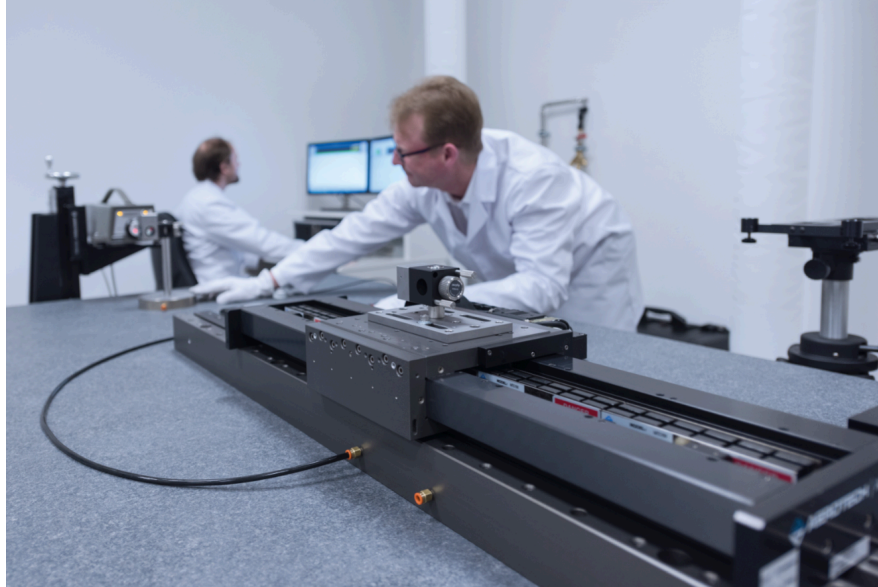
Figure 4. A technician performs metrology and calibration on a linear stage.
