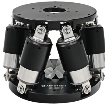
Figure 6. A hexapod's parallel-kinematic architecture typically increases stiffness and can save space.
